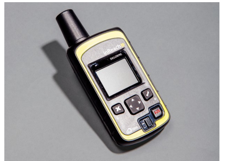
DeLorme's InReach SE is one of two devices we tested for sending texts via satellite. Photo by Ariel Zambelich/WIRED
